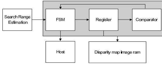
Figure 8. The hardware architecture of Error Correction.
