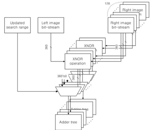
Figure 7. The hardware architecture of disparity estimation.
