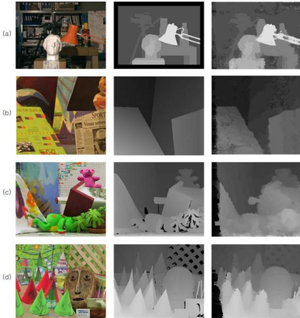
Figure 9. Disparity results of the proposed system. (Stereo pair(left), Ground Depth(middle), Proposed algorithm(right))
