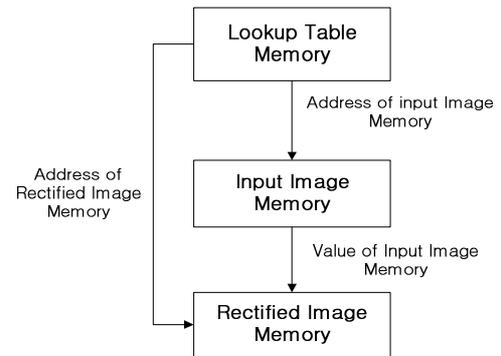
Figure 3. Flow of data transfer process
