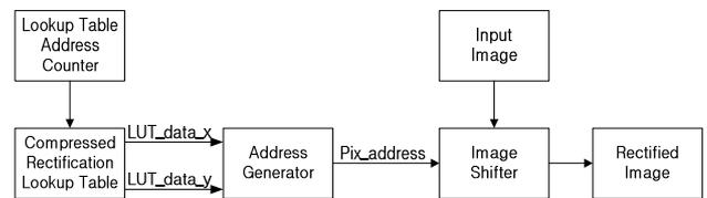
Figure 2. Structure of rectification module
