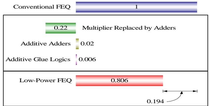
Fig-4 Power Reduction from Conventional FEQ to Low-Power FEQ
